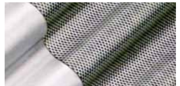
Vane fabricated with R0.75T1.5 pattern perforated material
